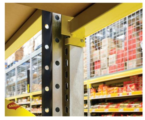
"Not only did we design the racking using a new yellow and silver colour scheme to ensure visual consistency across the stores; specialised tooling was also used to create a bespoke reverse punched upright and retail beam that would offer 25mm adjustment to all shelves (rather than the standard 50mm) for added flexibility," said Simpkin.
