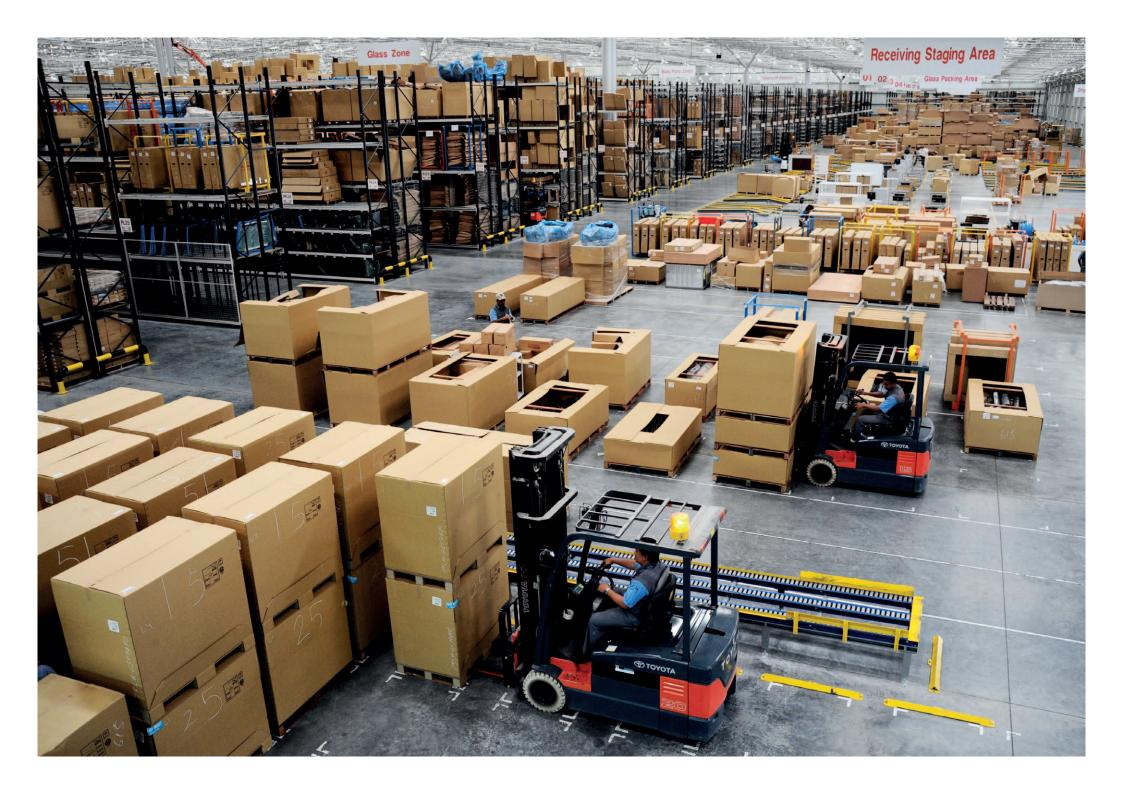
"The Dexion storage solution, supplied and installed by Famco, consists of more than 31,000 shelves enough to cover more than 7 football pitches and a total linear length of 54kms, 23,000 beams and 74km of uprights."
