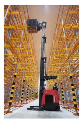
Dexion was awarded the project to design, manufacture, supply, deliver and install 10.2 meter high Double Deep racking system for the warehouse. The facility is located in VSIP Bac Ninh, one of the largest development of integrated industrial parks and mixed-use areas in Vietnam.
