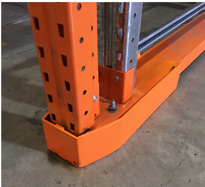
Custom Bull-nose Protector Plate using 5mm thick steel that would cover the front and a portion of the side of the floor channel.
